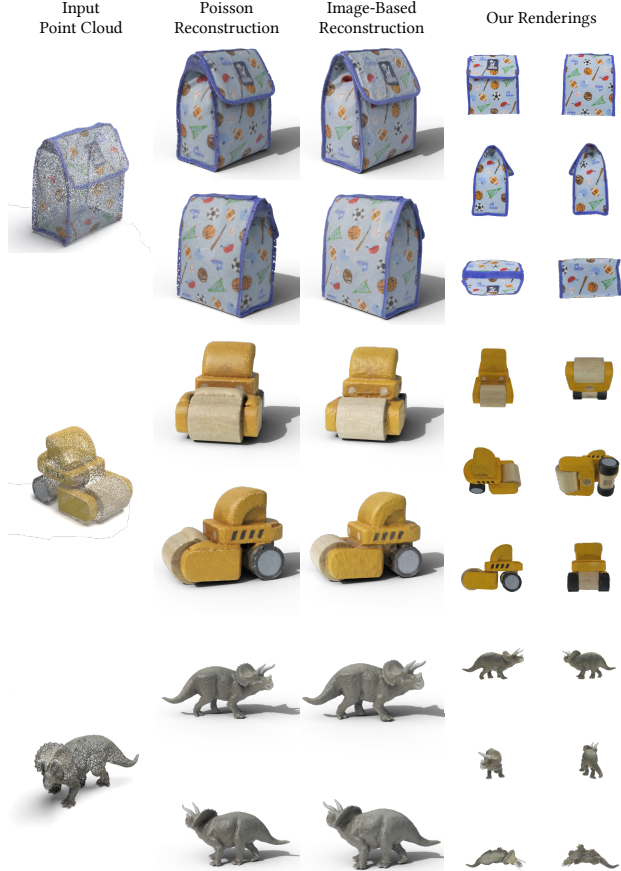
Figure 6. Visualizations of mesh reconstruction. Benefiting from the high-quality renderings, we utilize image-based mesh reconstruction algorithms to obtain mesh from input point clouds. Since our method bypasses some challenges, e.g., normal estimation, in some cases, our model produces mesh with better geometry and colors than Poisson reconstruction.
